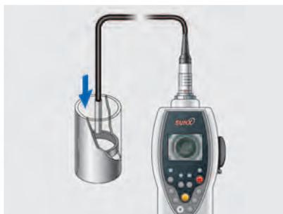
Inspection of the inside of metal parts
