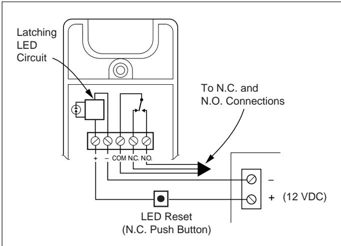
When the actuating lever is pulled between 20° to 45°, the alarm circuit switch (SPDT) will actuate. Then the LED will latch and light or change to red (3050), indicating that the SPDT switch has been activated. Closing the handle rearms the SPDT switch. However, the LED remains lit.
