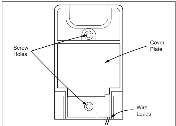
3. Drill pilot holes or start the screws. Connect the wire leads to the terminal block (see wiring diagram).
