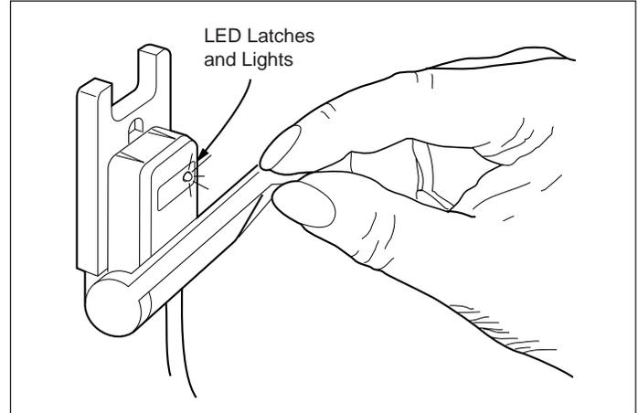
2. Close the handle. The SPDT switch is now fully re-armed. The LED remains lit.
