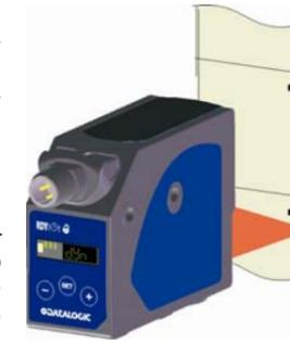
If the detection has been successful, the sensor returns to normal functioning. If it fails due to insufficient contrast, the 'FAIL' test blinks on the display. Press the (SET) push-button and the sensor returns to the previous setting.
